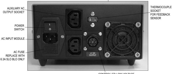
CONTROLLED LOW VOLTAGE DC OUTPUT
