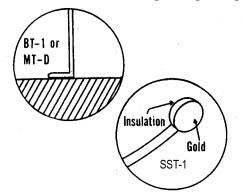
9.6. Straight probes may also be used, provided that sufficient shaft length is in contact with the surface to be measured. In general, the smaller the probe, the more accurately it will measure the surface temperature of a solid. For instance, an MT-29 microprobe, because of its small size, needs to be in contact with the surface for as little as 1/8". SST-1 has a 1/4" gold disc sensor. Gold is an excellent conductor, and is non-allergenic and non-polluting. It makes a fine skin surface probe.
