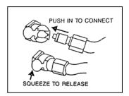
Connect one of the tubes from the OUTLET of pump to water INLET on the back panel of the controller.
