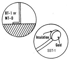
9.6. Straight probes may also be used, provided that sufficient shaft length is in contact with the surface to be measured. In general, the smaller the probe, the more accurately it will measure the surface temperature of a solid. For instance, an MT-29 microprobe, because of its small size, needs to be in contact with the surface for as little as 1/8". SST-1 has a 1/4" gold disc sensor. Gold is an excellent conductor, and is non-allergenic and non-polluting. It makes a fine skin surface probe.
