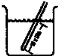
However, a liquid which has been heated above or cooled below ambient will be losing or gaining heat, and convection currents will give rise to temperature variations of up to several degrees. These variations can be reduced by vigorous stirring. This simple precaution must always be taken.
