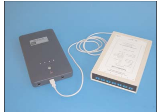
External Li-Ion battery pack powering Thermes Temperature Data Acquisition System
